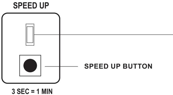
**Blinks** when panel is in speed up mode.
