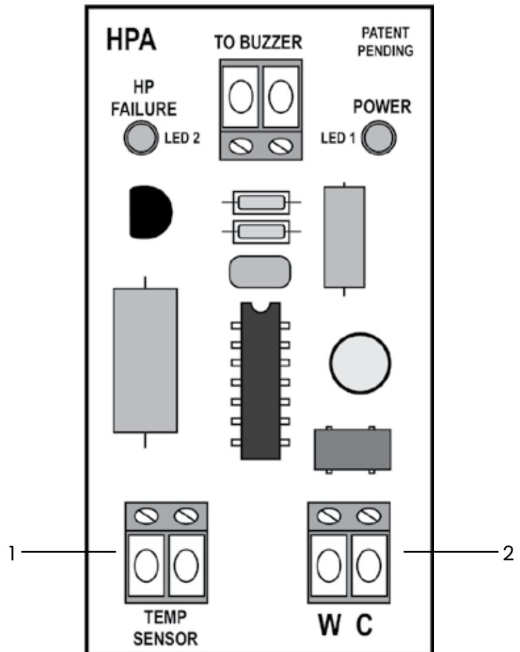
1. Temperature Sensor Input Terminals (N.O.)
