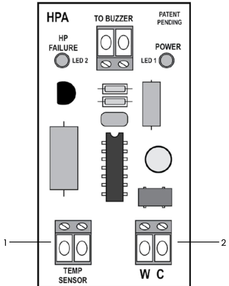
1. Temperature Sensor Input Terminals (N.O.)
