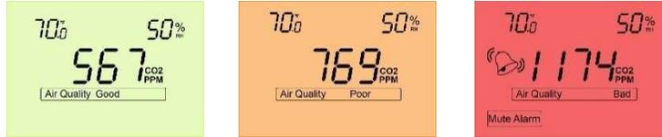
When enabled, user can mute an audible alarm by pressing the “Mute Alarm” button when shown. If Active Ventilation is enabled, the user can tap the “A” icon to briefly display the outside air temperature.
