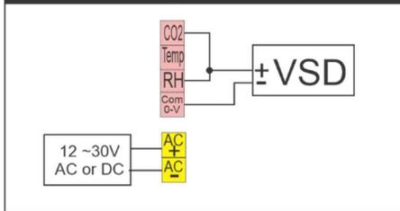
In this example the CO2 and RH is controlling the VSD with a high select. Both the CO2 and RH outputs are individually scalable so the CO2 range can be 450ppm to 1,000ppm and the RH range can be 75% to 100%. Also, the RH output can be limited to 7V max if required.
