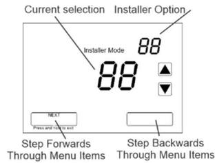
To advance through the menu items tap the “NEXT” button and adjust the shown installer option with the Up / Down arrows.
