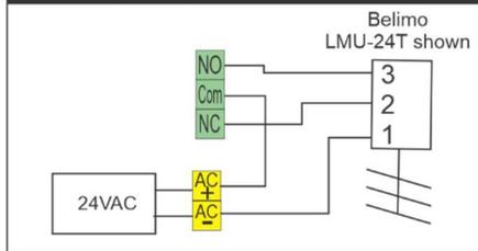
An open/close or an off/on output can be controlled by the monitor using the volt free relay provided. The relay threshold can be individually adjusted for each sensor. (30V @ 1A max)
