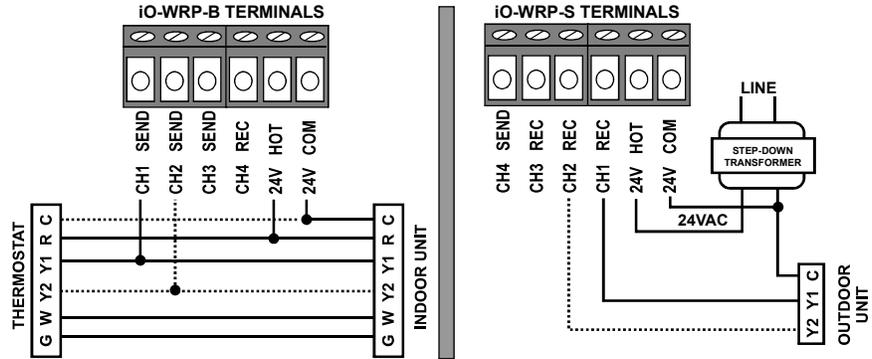
**HEAT PUMP UPGRADE WITH ONLY TWO WIRES TO OUTDOOR UNIT**
