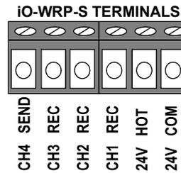
Please note the difference in terminal designations between the iO-WRP-B Base Module and the iO-WRP-S Satellite Module. The iO-WRP-B Base Module has three send and one receive channel. The iO-WRP-S Satellite Module has three receive and one send channel.
