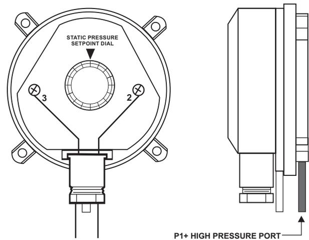
The Pressure Sensor should be mounted in a vertical position in an area accessible for wiring to the fresh air damper and attachment to the pressure tubing and probe.
